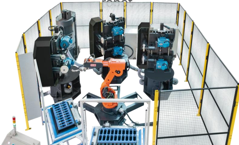
Sanitary equipment with YLM robot
